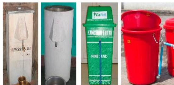
Figure 3: KAF versions developed over the years. (Left to right) concrete square, 2002; concrete round, 2003; plastic hilltake, 2003; plastic GEM505, 2004. Source: Ngai, 2005.
