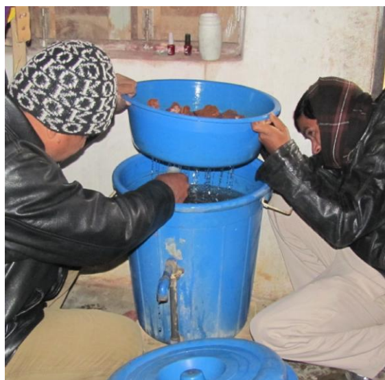
Figure 4: Collecting water sample after it has passed through the nails and is dripping from the diffuser basin into the sand layers. Hari Budhathoki (left) and Tirtha Raj Sharma Dhungana (right).
